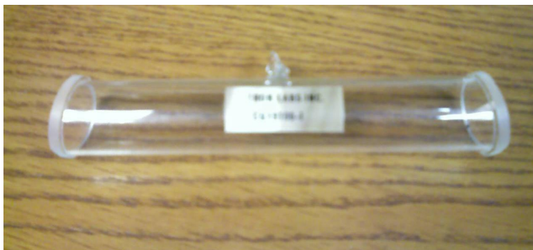
Figure 2.1: This cell containing I_2 gas was used in the saturated absorption spectroscopy setup. (Thorlabs CQ19100-I)
