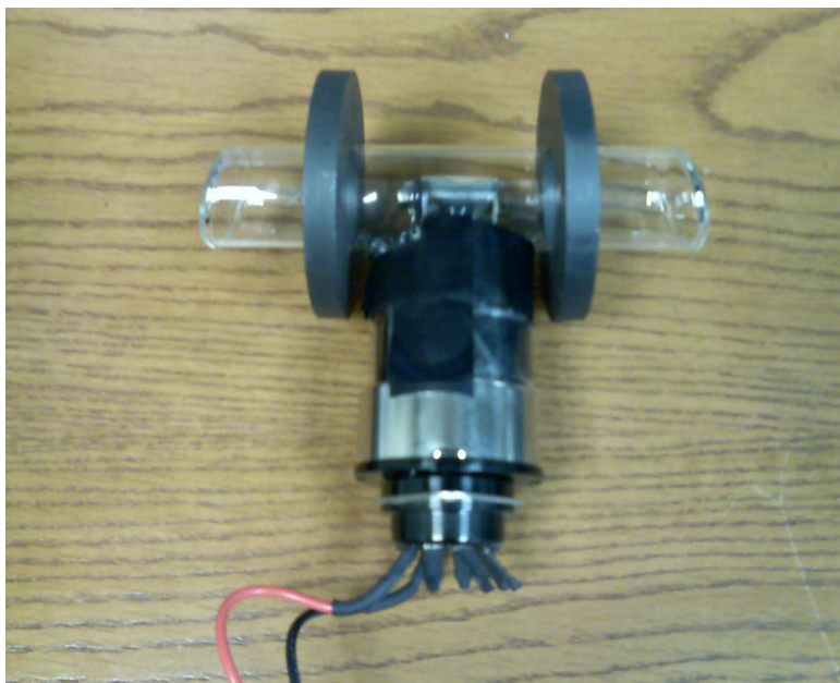
Figure 3.2: The hollow cathode lamp used in the DAVLL setup. Shown also are two of the six ring magnets used to provide the B field.
