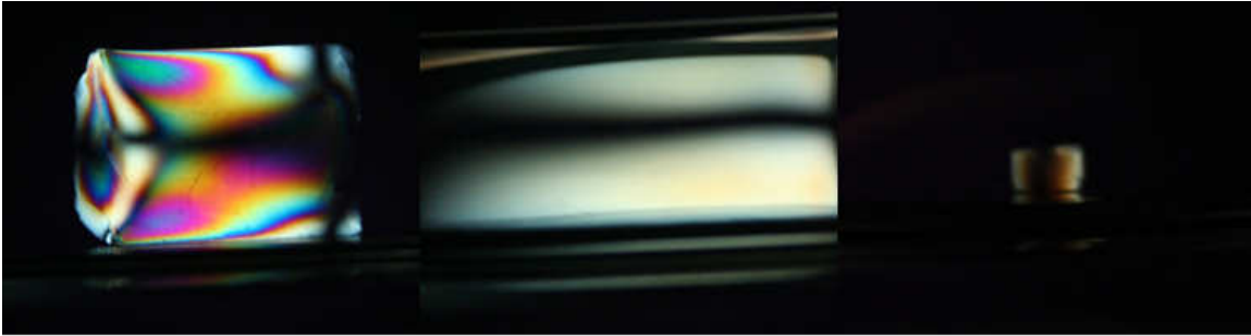
Fig. 6 - From left to right: an aerogel sample exhibiting both local density variations and anisotropy, an aerogel with inhomogeneously distributed anisotropy, an aerogel with an isotropic core and anisotropic surroundings
